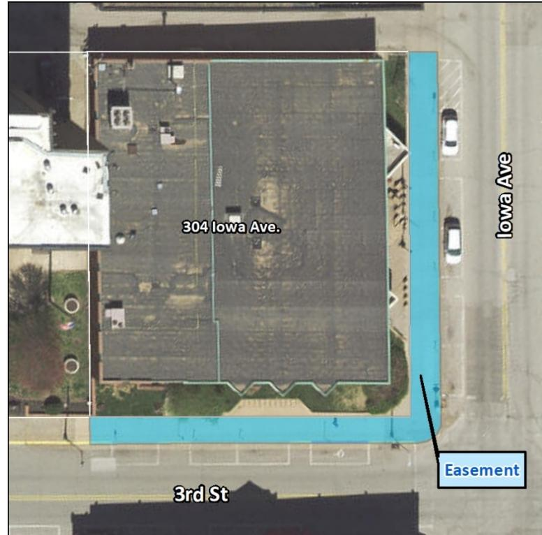
In order to facilitate better stormwater management, the Stanley Center is requesting to make alterations to the public sidewalk along the northeast and southeast fronts of the property along 3<sup>rd</sup> Street and Iowa Avenue. Work will include removal and replacement of sidewalk paving, installation of permeable pavers, installation of trees and tree grates within sidewalk;
