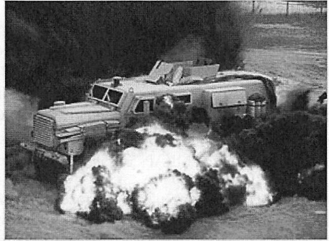
An MRAP Cougar HE tested in January 2007, with landmines detonating around it.
