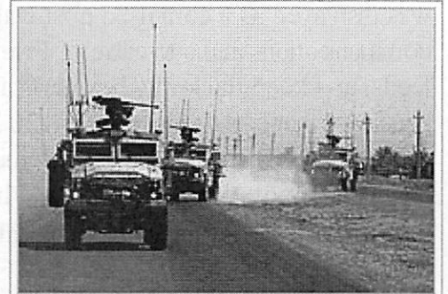
A RG-33 convoy with the Common Remotely Operated Weapon Station (CROWS) system installed.
